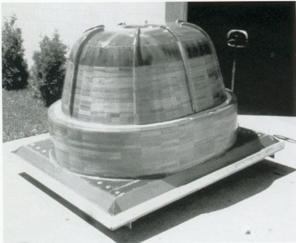
Hampel Corp. recently formed a part using this 40-inch-deep male wood pattern, 58 inches in diameter.
